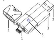
Lightning cap open mode: Turn the cap gently to pull it out.
